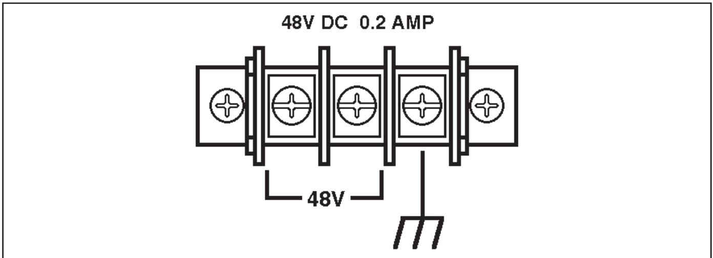
Figure 4.1: Terminal Block Assembly (DC Units Only)
