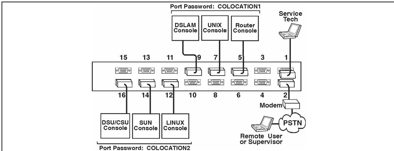
Figure 4.2: APS Application Example (Model APS-16 Shown)
