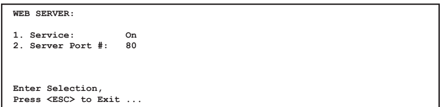
Figure 5.15: Web Server Parameters Menu - Text Interface
