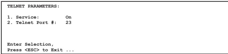
Figure 5.13: Telnet Parameters Menu - Text Interface
