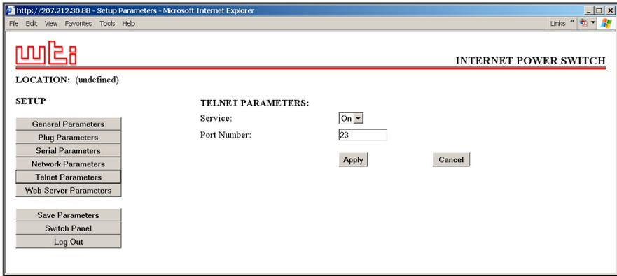
Figure 5.12: Telnet Parameters Menu - Web Browser Interface
