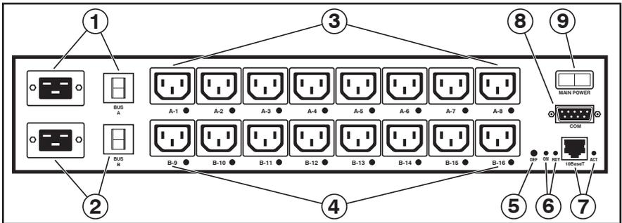
Figure 2.2: IPS-1600CE-D16 Back Panel (16-Plug Unit)
