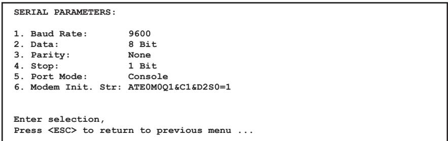
Figure 5.6: Serial Parameters Menu - Text Interface
