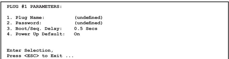
Figure 5.8: Plug Parameters Menu - Text Interface (Plug 1 Shown)
