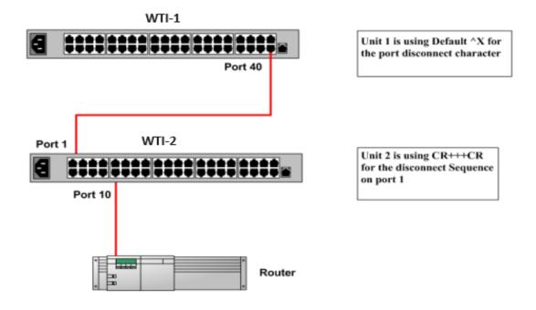
Set the Logoff character to "+" symbol and Sequence Disc to Three Chars on port 1 of WTI-2. This will allow you to maintain command mode presence in WTI-2 and not disconnect you all the way back into WTI-1.
