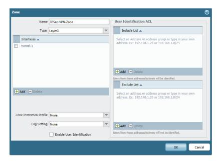
You need to define a separate virtual tunnel interface for IPsec Tunnel. To define the tunnel interface, Go to **Network** >> **Interfaces** >> **Tunnel**. Select the **Virtual Router**, an *IPsec-VR* in my case. Also, in **Security Zone** field, you need to select the security zone as defined in Step 1.
