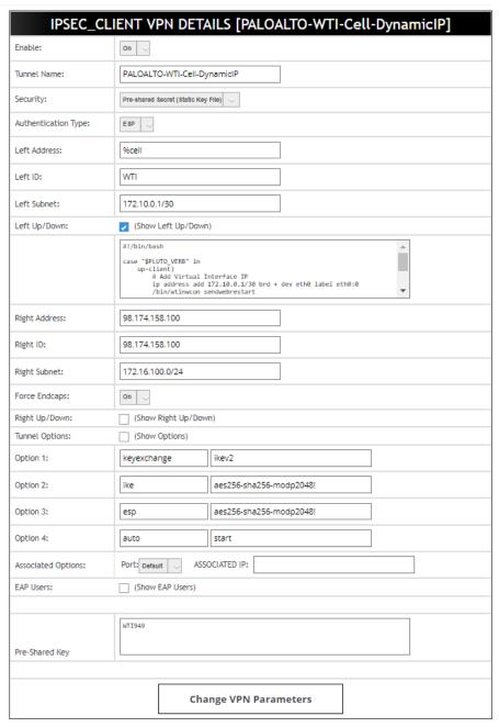
**Note:** Use the static IP as the left address for the static IP address on the Cell interface. Alternatively, use %any for the left address to allow the VPN tunnel from any interface (eth0 or cell).
